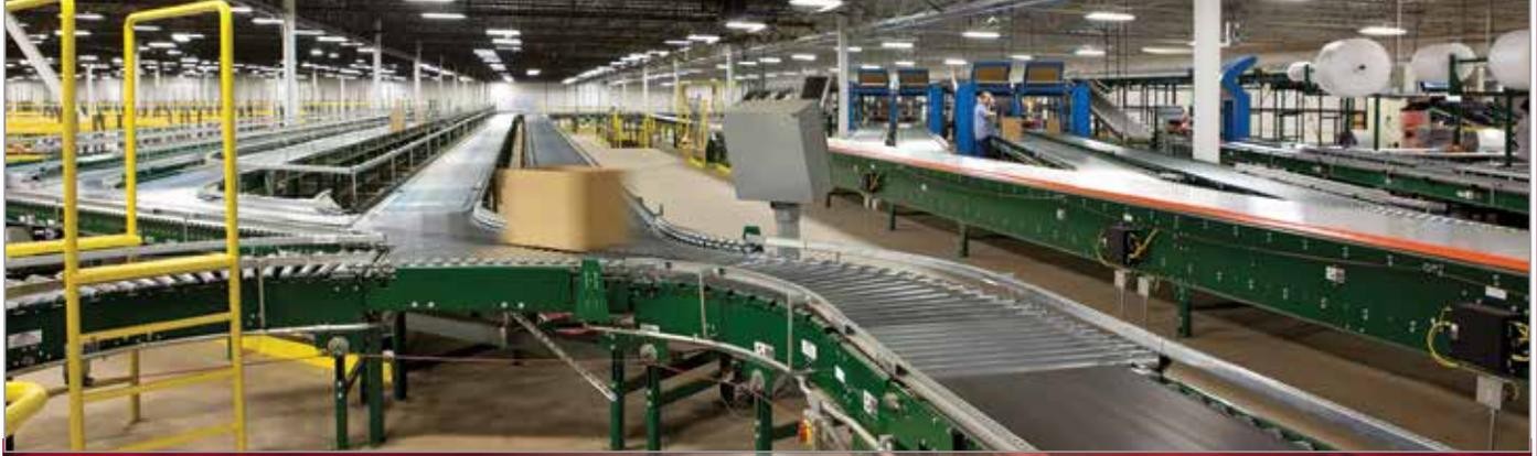
*The Atlanta facility can expand by another 250,000 square feet if necessary, includes 2.5 miles of conveyor, and a shipping sorter that can travel at 684 feet per minute, sorting up to 9,000 cartons per hour.*
